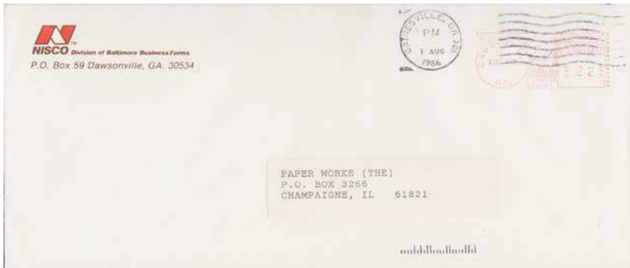
Figure 34. Fragmentary barcode showing the right side of the POSTNET barcode (left side will be found on the other envelope presumably addressed to Aurora IL 60506): 60506 (3) is deduced from these bars.
