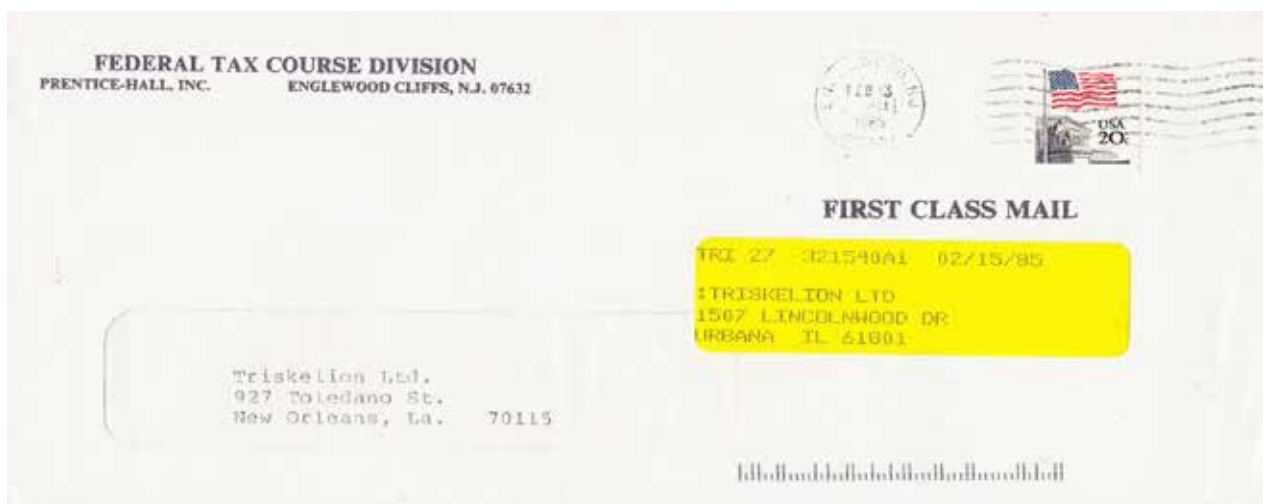
Figure 33. Double feeds can cause completely wrong POSTNET codes: 60568-0001 (4) This barcode represents the unrelated envelope that was imaged in front of this cover. (The addressee on this envelope happened to have moved and therefore a yellow Computerized Forwarding System label was later applied as the envelope was forwarded from Louisiana to Illinois.)
