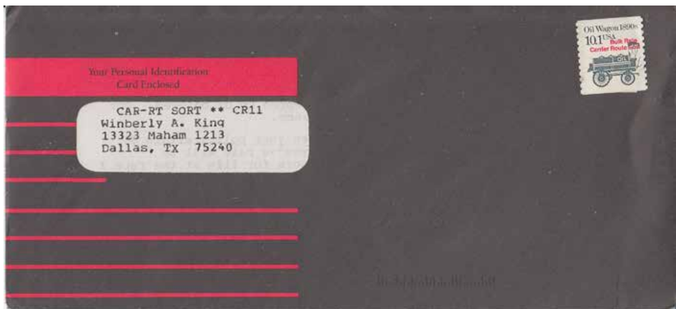
Figure 31. Black envelope with a POSTNET barcode: 75240 (2) which could not be read by the contemporary barcode reader. The barcode is faintly visible at the bottom center in the scanned image.
