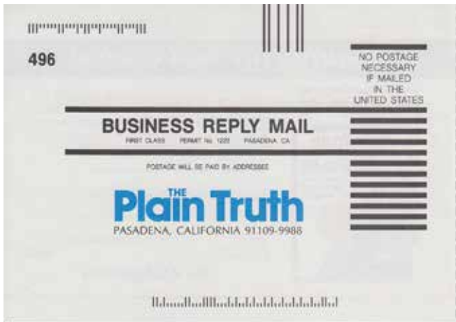
Figure 30. POSTNET barcode at the bottom and intentionally inverted internal corporate barcode in the upper left for internal sortation purposes.
