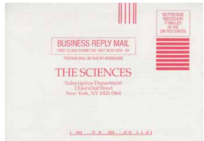
Figure 13. Red POSTNET barcode on preprinted business reply card violates the USPS color specifications.
