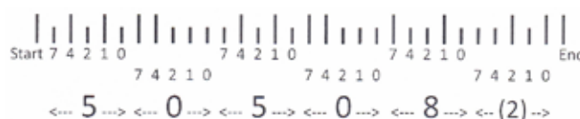
Figure 8. Decoding a 5 digit (32 bar) POSTNET barcode
