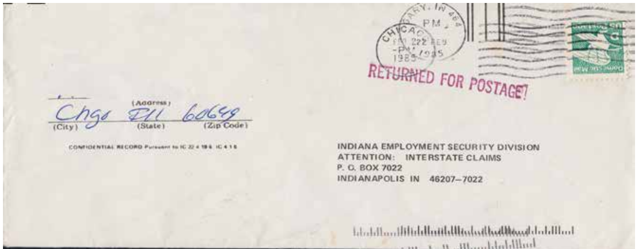
Figure 27. Multiple POSTNET barcodes: 46207-7022 (0) (3 times).
