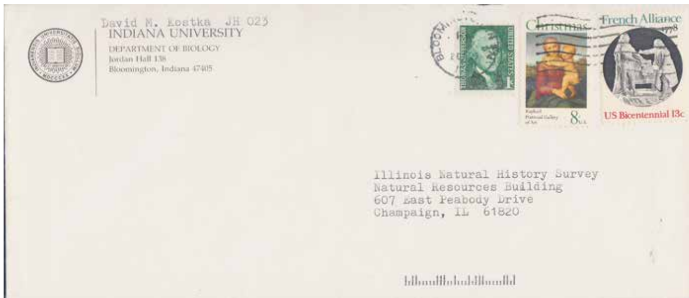
Figure 3. Five digit ZIP coded envelope with matching POSTNET barcode: 61820.
