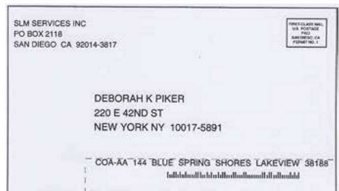
Figure 17. USPS sample FASTForward envelope from USPS Postal Bulletin 21943 (April 10, 1997). If the addressee moves, the corrected address and POSTNET barcode are printed by the MLOC system in the lower right corner of the envelope.
