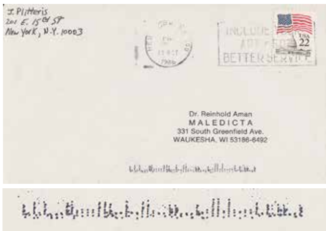
Figure 24. Poorly adjusted printer damages POSTNET barcode: 53186-6492 (6).
