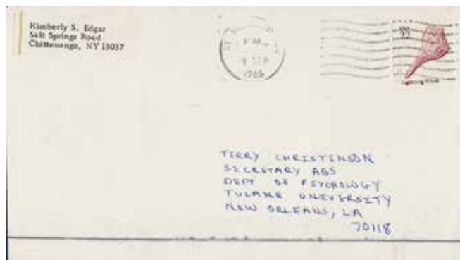
Figure 15. Solid black line associated with misadjusted POSTNET barcode printer.
