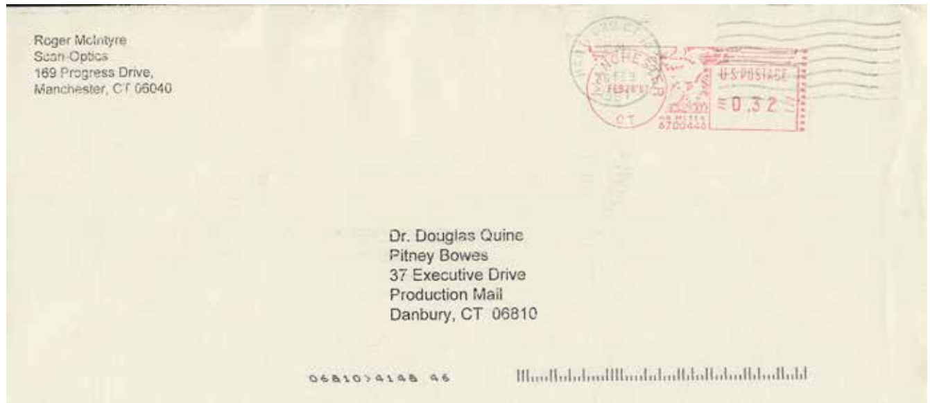
Figure 16. Human readable text 06810>4148 46 to left of USPS printed POSTNET barcode representing the 5 digit ZIP, ">" symbol, +4 digits, and the carrier route number.
