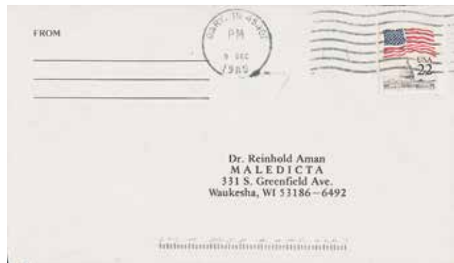
Figure 25. Poorly adjusted printer loses readability of tall POSTNET bars, as they are missing detail.
